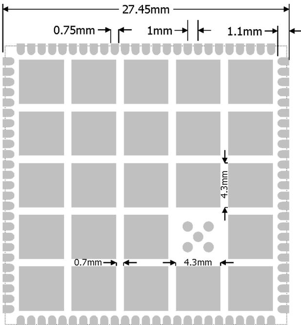
The ground pad solder mask on the bottom side of the QSCOM module is divided into sections for a better reliability of the solder joint and self-alignment of the component.
